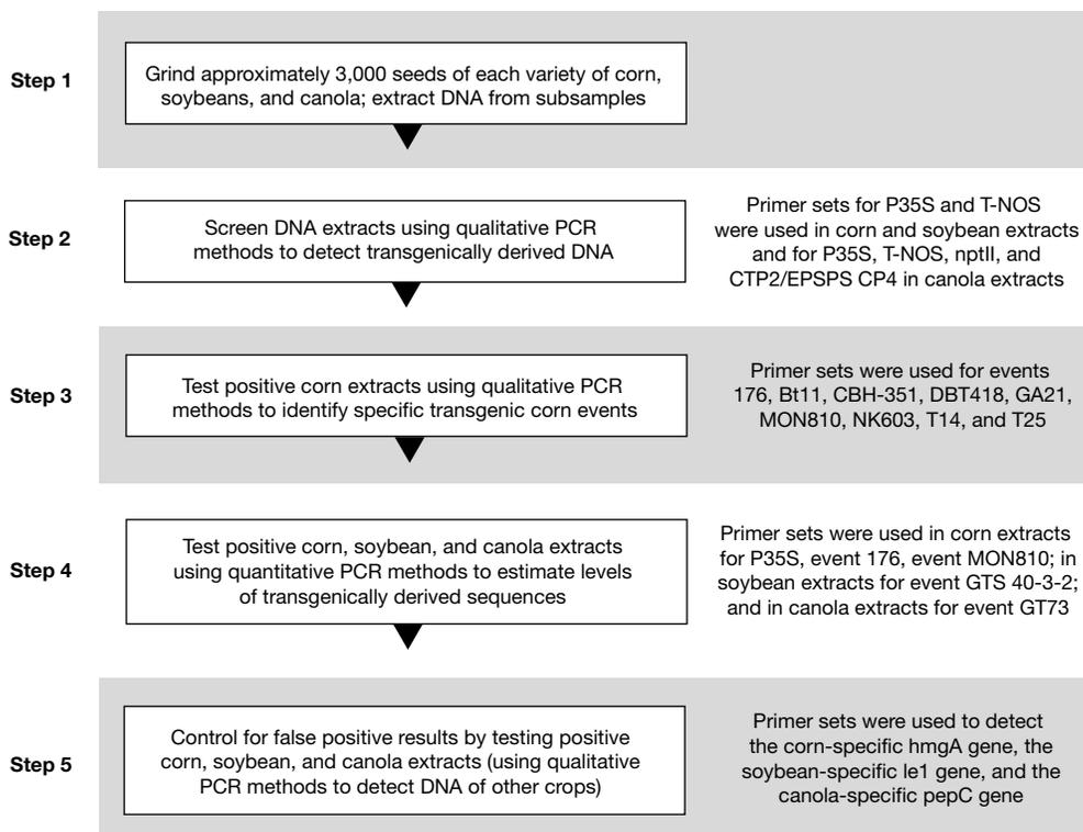
*Detecting transgenically derived DNA.* The laboratory ground approximately 3,000 seeds<sup>38</sup> of each variety, extracted DNA from a subsample of the ground material, and used qualitative PCR methods to screen DNA samples. As shown in Figure 2-1, Step 2, primer sets for P35S and T-NOS were used to screen corn and soybean samples, and P35S, T-NOS, nptII, and CTP2/EPSPS CP4 were used to screen canola samples (at a detection limit of approximately 0.1 percent<sup>39</sup>).
